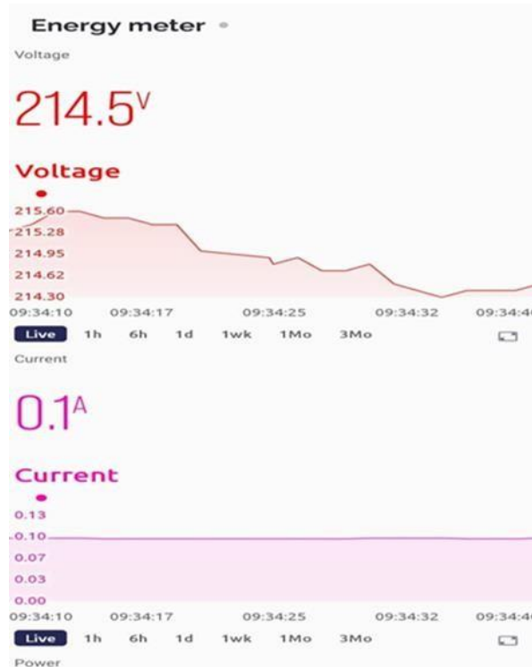
Fig. 7 Representation of total voltage, total current that overall appliance consumed.
